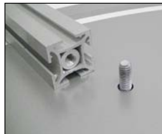
Base Plate Connection
